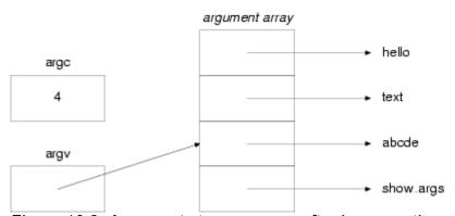
Figure 10.2. Arguments to a program after incrementing argv
