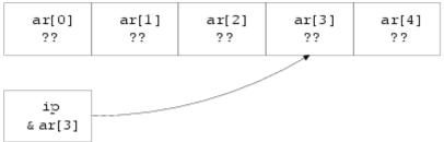
Figure 5.4. Array and initialized pointer
